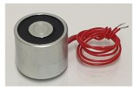
This magnet exerts a holding force of approximately 12 Kgf perpendicular to any steel plate (see accessories) with which it is in contact, assuming nominal voltage, and coil at working temperature rise of 60°C in an ambient of 20°C.
